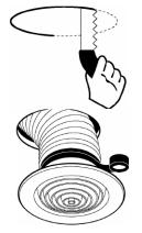
Ensure there are no obstructions above the ceiling in the selected location. Using the template provided, mark hole for the grille:
