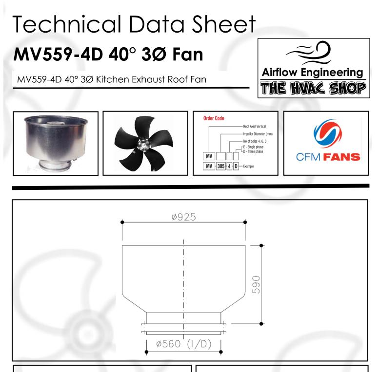
MV models are high-capacity roof mounted axial exhaust fans they are kitchen exhaust fans. The all-metal fan casing provides a long lasting and robust construction. Suitable for high temperature kitchen exhaust systems. Motor: 415V 50Hz 3 Phase 4.6 Amp Full Load Current 1440 RPM Total Motor Wattage 2.2kW Aerofoil adjustable pitch impeller Performance tests are in accordance with BS848 Part 1 (1980) and AS2936 – 1987 Impellor Diameter: 559mm diameter
